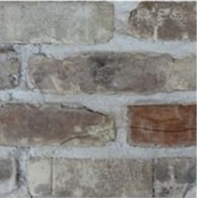
Type: Used bricks (whole and half) Thickness: 108 mm Density: 1800 kg/m³ Lifetime: Not listed EPD no: MD-16007-EN
